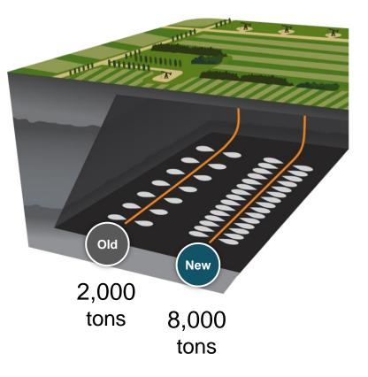
More proppant = the quickest and cheapest way to increase well output
