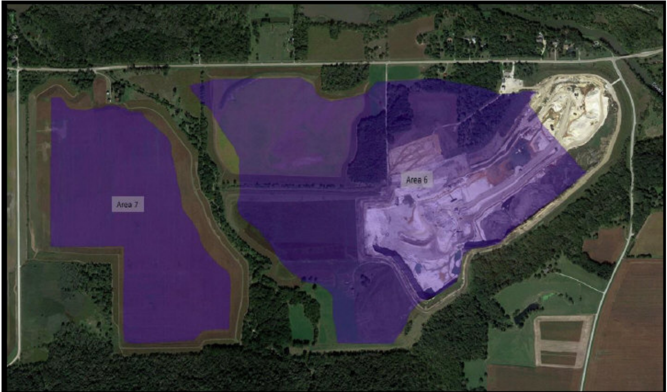
Figure 15.4 - Possible tailings storage pond locations in the South Ottawa and West Pit areas.
