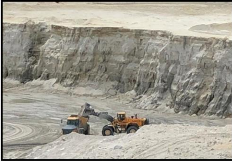
Figure 13.3 - A front-end loader loading blasted sandstone into an articulating haul truck.
