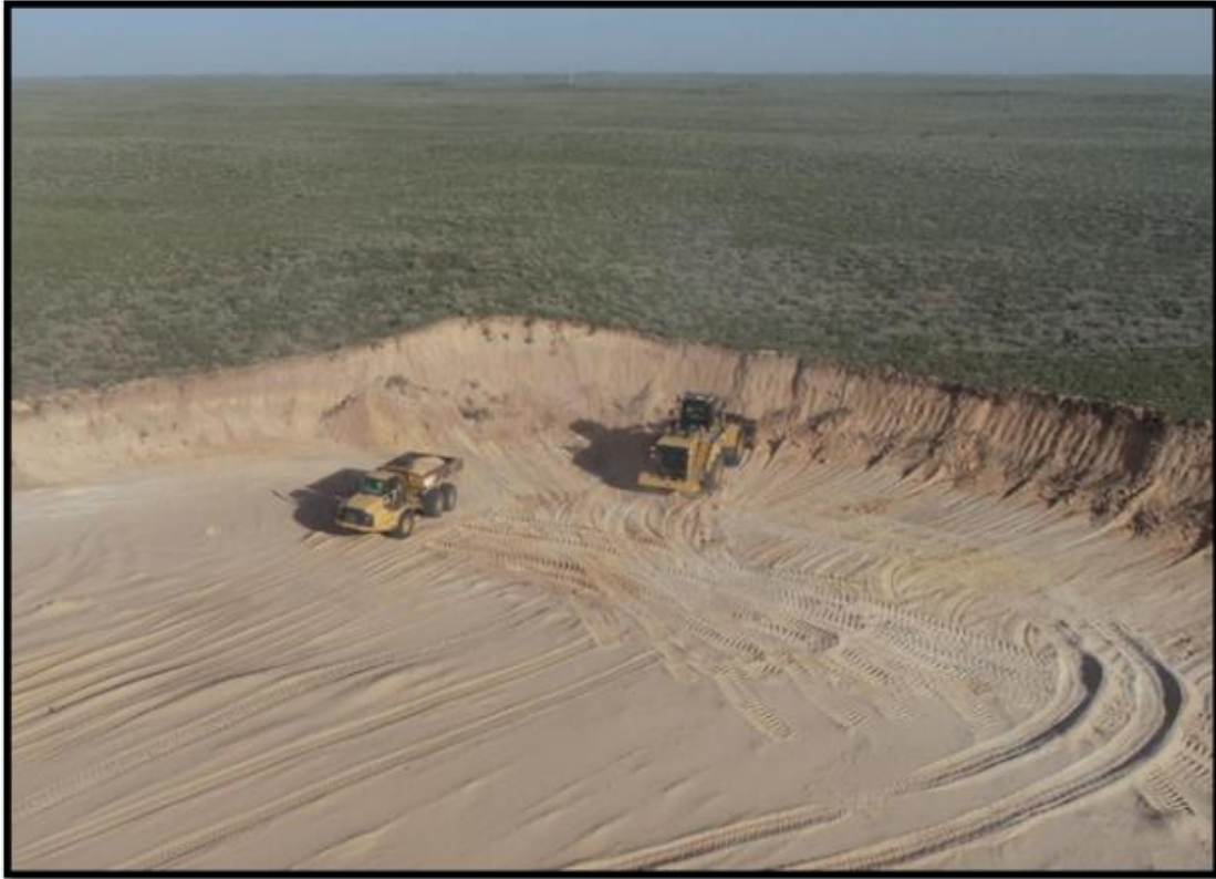
Figure 13.3 – Typical mining operation at Lamesa showing a front-end loader excavating the full bank section of overburden, the “Upper Clean Sand,” and the Clayey Cover Sand.
